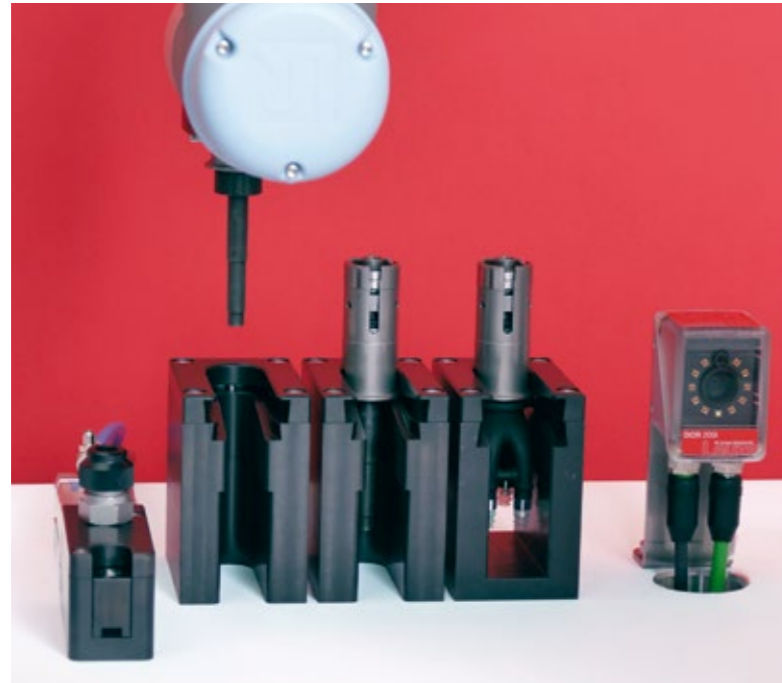
From left to right: external supply unit, 3x tool station, encoder
