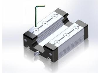
First, if necessary, adjust the sliding of the carriages on the linear bar by acting on the screws on the carriage itself. Turning clockwise, the rigidity and the precision of the arm will increase. Kolver provides pre-calibrated screws at 0.55 Nm.
