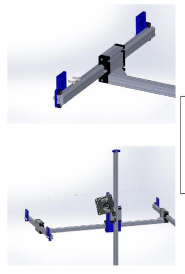
On XYZ model, fix the lateral bars with relative screws at 877 mm from each other to allow the assembly of the horizontal bar.
