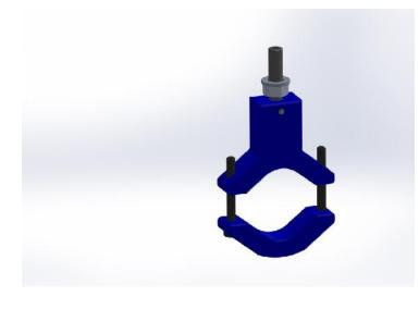
To secure the support of carbon bar, screw the threaded socket and lock the rotation with the nut.
