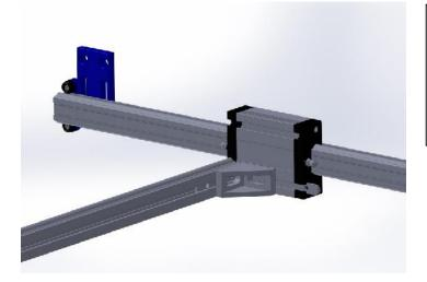
Place the horizontal bar as shown in figure holding the bracket parallel to the carriage, insert the threaded nuts and fix both sides.
