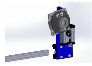
After removing the limit switch, insert the horizontal bar on the appropriate guide of the carriage.
