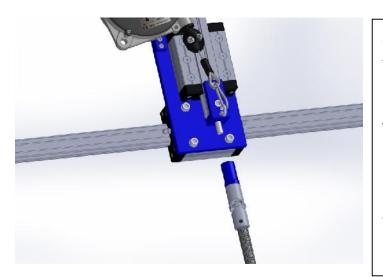
Screw the rod bush of the carbon bar on the threaded pin and secure it with a 18mm wrench.
