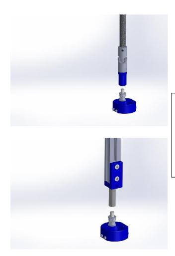
Screw the clamp in the aluminum bush for at least 5 mm, find the desired position and tighten nut + washer to lock the rotation.
