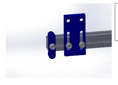
Adjust the screws on the rails in order to give the desired tilt to the bar and, once released the screwdriver, the carriage can slide to the default position.
