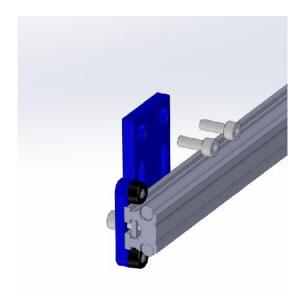
Place the supports to fix the system on both sides of the horizontal bar.
