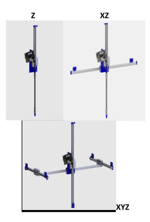
The new Suspended Torque Arms are the ideal solution to increase productivity. They can be easily installed on most work stations to help the operator handle the screwdriver in total safety and stability. With minimized reaction force you will also improve finished product quality because there is no movement of the tool and all torque is absorbed in the joint. They also improve the comfort of the operator and the productivity clearing the work area and maximizing use of the space.
