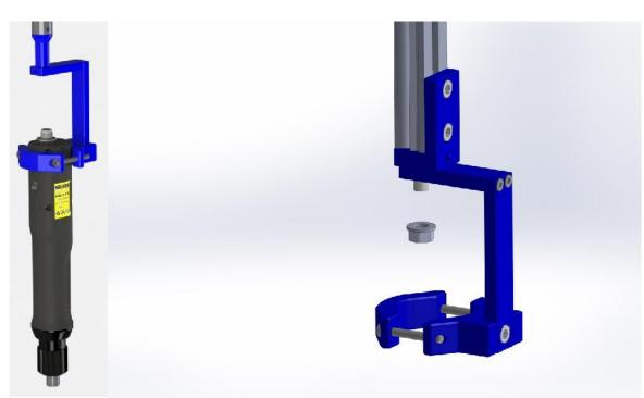
To secure the universal clamp on the carbon bar, tighten the screw M8 x 20 on the bush bushing and fix the M4 nut to prevent unscrewing. To secure the support of XYZ model, screw the M8 nut + washer on the threaded pin of the vertical bar.
