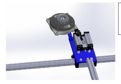
Remove the limit switch (see point 2) and insert vertical bar (see point 4). Reassemble the limit switch.
