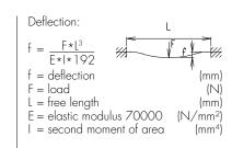
For the diagram for critical speeds of lead screws refer to chapter 4.2
