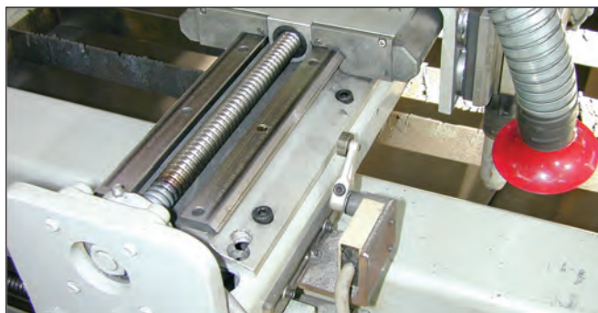
This multi-axis plasma cutter, using a LoPro ball screw driven system, operates in a harsh environment consisting of smoke, abrasive dust, weld splatter, hot sparks and elevated temperatures.
