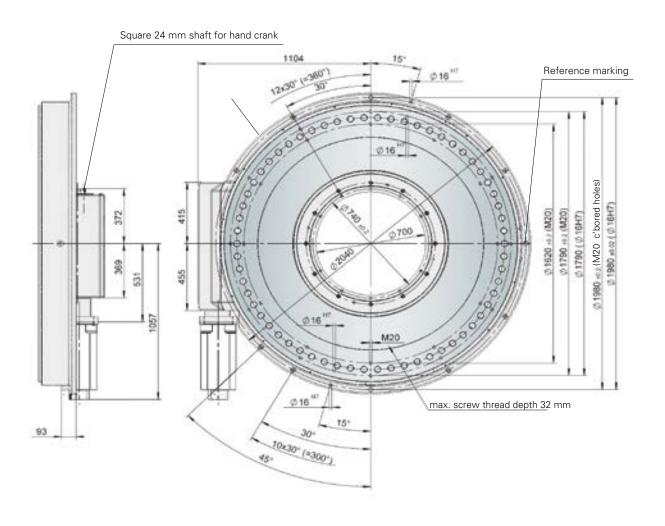
The shown position of the dial plate corresponds to the home position (state of delivery). The motor dimensions refer to the model 8LSA84.E1022D200-0 by B&R. It is possible to fit alternative motors from various manufacturers. An additional reduction gear may be required with several motors.
