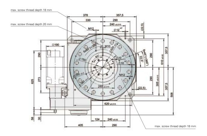
The shown position of the dial plate corresponds to the home position (state of delivery). It is possible to fit popular alternative motors from various manufacturers.
