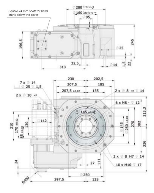
It is possible to fit popular alternative motors from various manufacturers. The drive flange geometries are motor-dependent. A taller central section is available on request.
