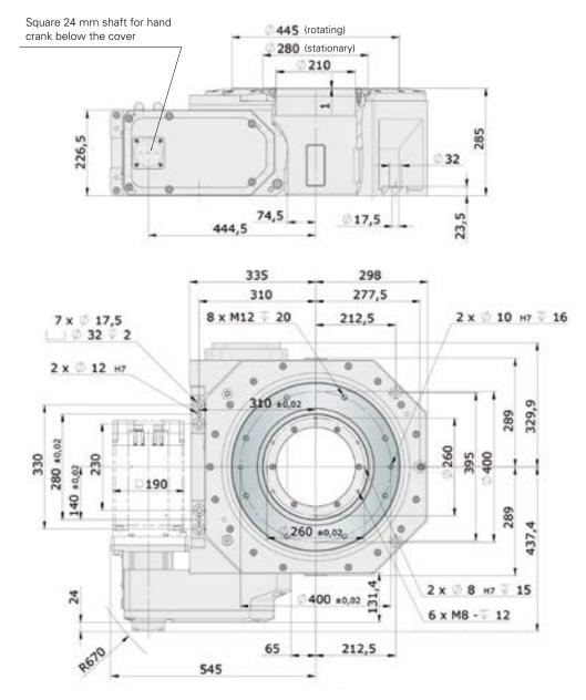
It is possible to fit popular alternative motors from various manufacturers. The drive flange geometries are motor-dependent. A taller central section is available on request.
