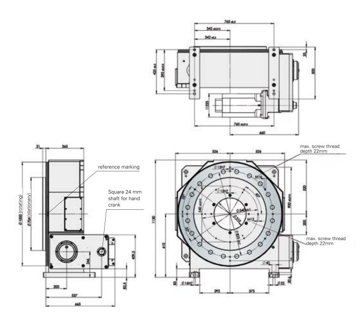
The shown position of the dial plate corresponds to the home position (state of delivery). It is possible to fit popular alternative motors from various manufacturers. The drive flange geometries are motor-dependent.
