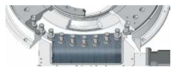
This cooling carousel at one of Cirey's casting stations in the Netherlands has a diameter of 10 metres and weighs 30 tonnes. It is driven by a CR. A special bearing has been fitted to handle the high breakdown moment as a result of the uneven load.
