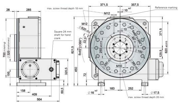
The shown position of the dial plate corresponds to the home position (state of delivery). It is possible to fit popular alternative motors from various manufacturers. The drive flange geometries are motor-dependent.
