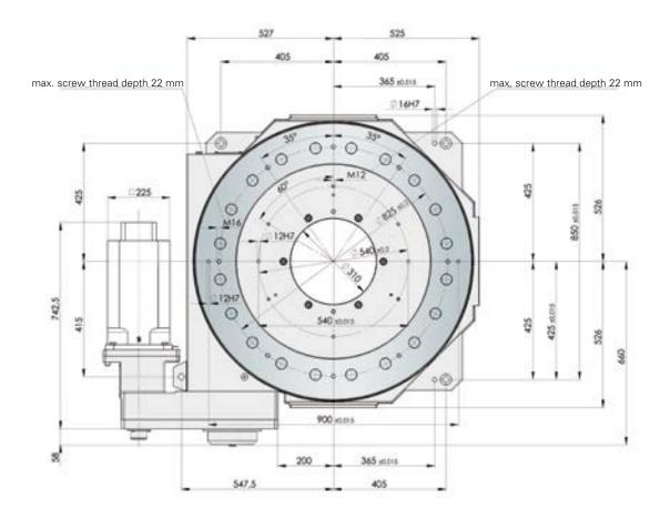
The shown position of the dial plate corresponds to the home position (state of delivery). The motor dimensions refer to the model 8LSA84.E1022D200-0 by B&R.
