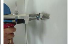
The operator presses the PHS onto the screw location and pushes the release button.
