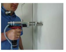
The operator pulls the PHS back. The next screw is immediately blown into position.
