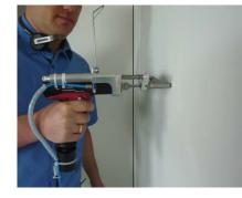
The screw is fed into the PHS. When the screw has reached its position it is firmly protruding from the nose piece. Thus it is held in position and can't be pushed back into the nose piece.
