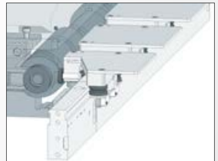
Linear Assembly System LS280 consisting of four assembly cells with locking station and base frame, as well as of belt sections, corner units and workpiece carriers.
