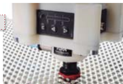
Ejector EMM integrated into gripper housing for Delta robots with Varioflex® bellows vacuum cups and workpiece
