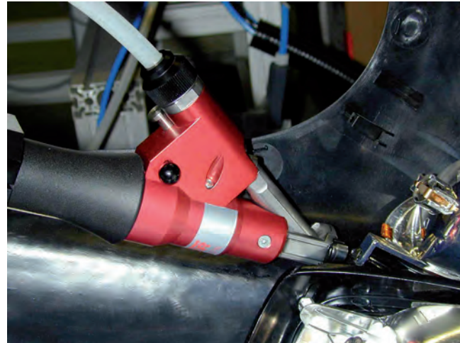
Fitting headlights in motor scooter fairings
