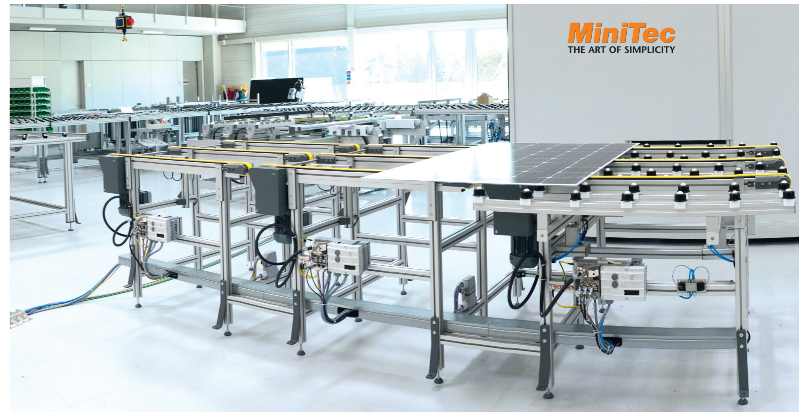
Solar Line with Flasher Unit
