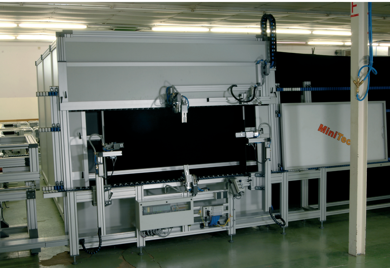
Module flasher with integrated HV-test/isolation test
