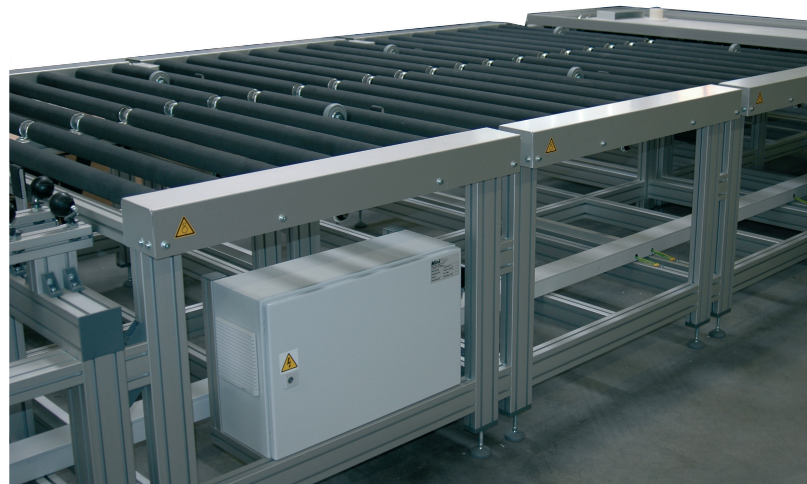
Roller conveyor with mechanical accumulation protection
