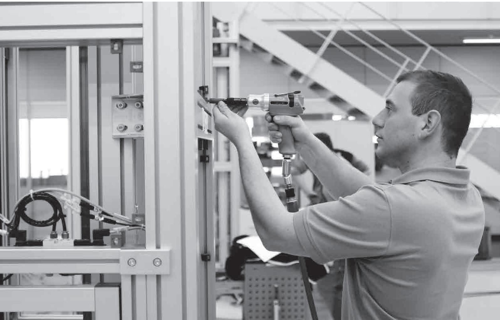
Compressed air is often used in the workplace systems for the operation of pneumatic cylinders in mounting devices or for the drive of compressed air tools. In order to minimize contamination at the workplace and to keep the health burden on employees as low as possible, one should always try to work with clean and dry compressed air.
