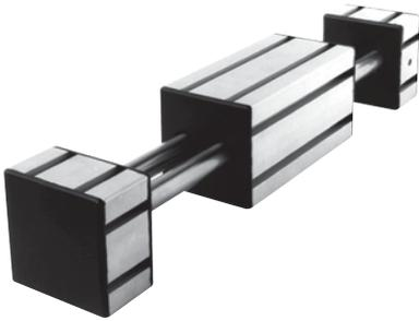
The LB design is based on LME 20 linear ball bearings that are built into our construction profile in the specially provided bore holes. Precision shafts D 20 mm provide the high load capacity of this guide. The LB design offers substantial advantages for short travelling distances and high stroke frequencies.
