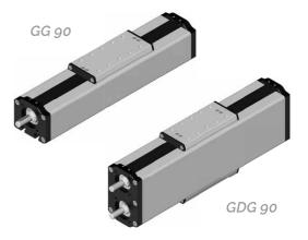
The guide bodies of our positioning systems consist of aluminium square profiles with edge lengths of 90 mm; the carriage inside the square profile is driven by a spindle with a corresponding lead nut.
