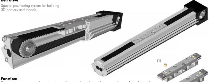
The guide body consists of an aluminium profile with elegantly rounded outer edges, with a roller guide integrated into it. The carriage is moved by means of a revolving interior timing belt. At the front face there is a timing belt deflection unit with integrated coupling claws on two sides. The opposite front face is provided with a plate containing a tensioning device for the timing belt.
