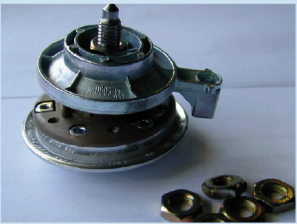
Fitting nut to drum bearing
