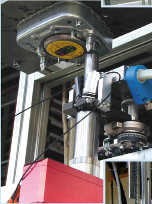
Attaching air bag assembly, vertically from below
