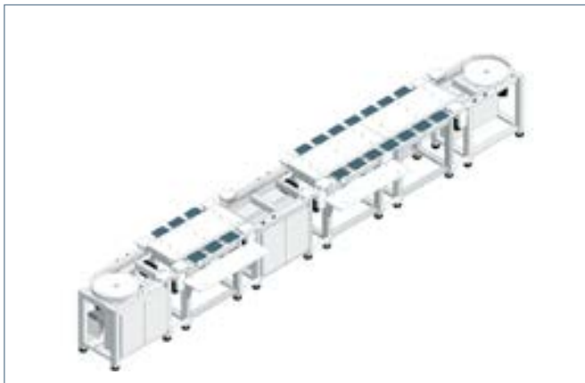
Example of 180° system layout
